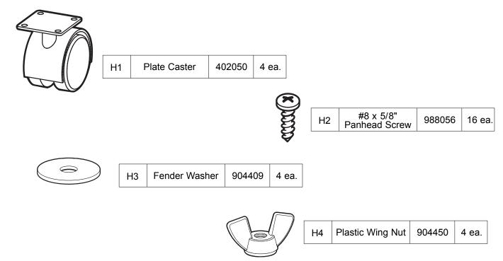
Place the Bottom Panel (A) on a clean, carpeted surface with the pre-drilled holes facing up. Attach four Plate Casters (H1) to the underside of the Bottom Panel using the #8 x 5/8" Panhead Screws (H2) in the pre-drilled holes as shown.
