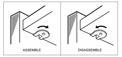
Place the Top (C) Divider (H), Storage Shelf (E), and Keyboard Shelf (K) on a clean, carpeted surface as shown. Tap in Rafix Cams (H1) into each panel where indicated with the flat edges aligned.
