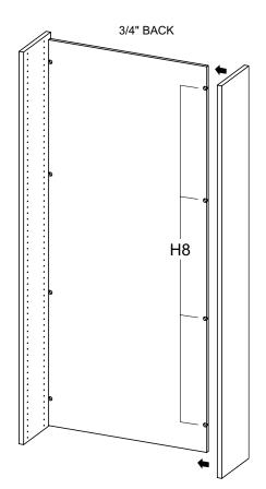
Turn Rafix Cams (H8) 1/2 turn clockwise to tighten.
