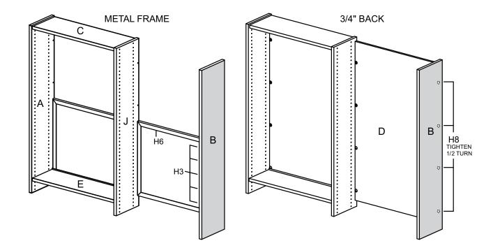
Assemble the Top Panel (C) and the Fixed Shelf (E) to the unit as shown. Lock the Tab-V Cams (H1) to secure the parts in place.
