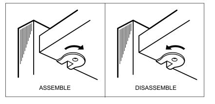
Install four Rafix Shelf Cams (H5) into each adjustable shelf. Attach a Book Stop (H2) to each Fixed/Adjustable Shelf (E) using five Panhead Screws (H3) in the pre-drilled holes.
