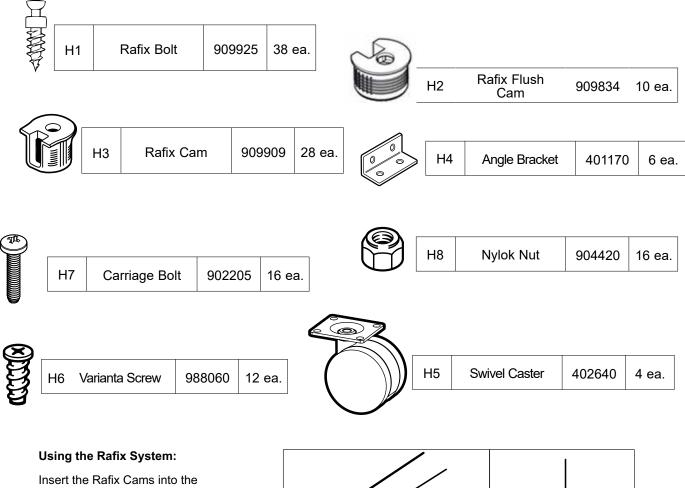
Insert the Rafix Cams into the appropriate holes. The flat edge of the cam should be facing the edge of the panel.
