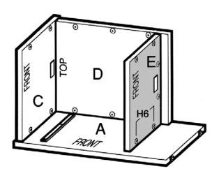
Secure the Fixed Shelf (E) to the Back (D) by turning the rafix cams.
