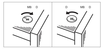
Insert four Minifix Cams (H1) and screw four Minifix Bolts (H2) into the Top Panel (C) as shown.
