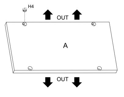
Fit the Sides (A) over the Rafix Bolts (H3) already installed on the Bottom (E). Using a Phillips screwdriver, rotate the Flush Rafix Cams (H4) clockwise to secure in place.
