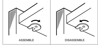
Place the Bottom Panel (E) face down on a clean, carpeted surface with the pre-drilled holes facing up. Install four Plate Casters (H1) at each corner of the Bottom using Panhead Screws (H2) in the pre-drilled holes as shown.
