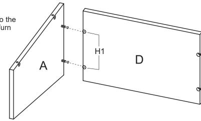
Position the Lectern Side (B) onto the Left Lectern Back (D) and turn the cams (H1) to secure.
