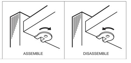
Place the Lectern Back (D) on a clean, carpeted surface or foam padding with the cam holes upright as shown. Insert eight flush rafix cams (H4) into the Lectern Back where indicated.
