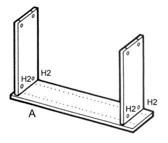
Position the Right Side (B) over the partially assembled unit insuring the Steel Posts are inserted into the corresponding Cam Devices (H2) as shown. Rotate the Cam Devices clockwise to tighten.
